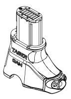
The TASER CAM recorder is an audio-video recording device integrated into a rechargeable X26 power supply that replaces the standard DPM battery pack and is compatible with all X26 ECDs. The TASER CAM recorder is activated any time the safety switch is in the up (ARMED) position. This allows officers to capture vital information prior to, during, and after the deployment or potential deployment of the X26 ECD.
