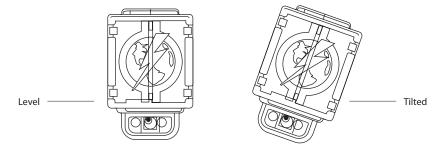
For most deployments, hold the ECD level. Do not tilt the ECD unless it is necessary to do so to align the ECD with the target.
